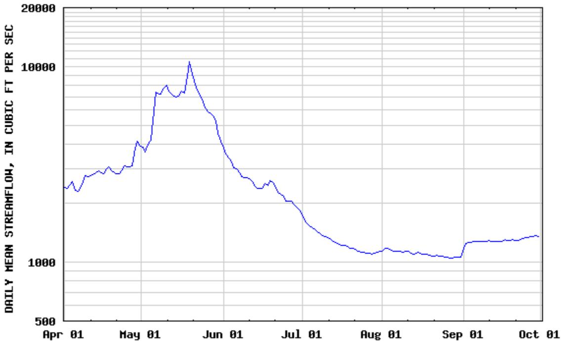
**Figure 25. Daily mean stream flow (Ft<sup>3</sup>/sec) from the Klamath River at the Seiad USGS flow gauge from April to October, 2005.**
