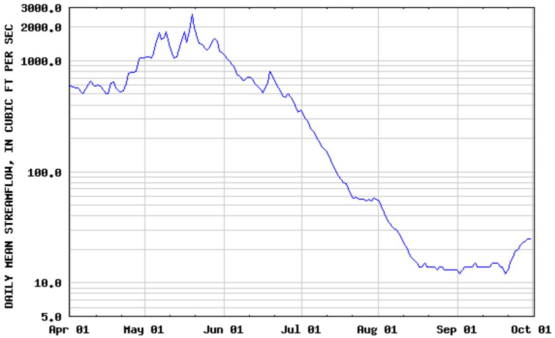
Figure 24. Daily mean stream flow (ft<sup>3</sup>/sec) from the Scott River at the Fort Jones USGS flow gauge from April to October, 2005.
