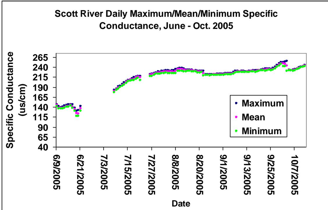
Figure 20. Daily maximum, mean, and minimum specific conductivity in the Scott River from June to October, 2005.
