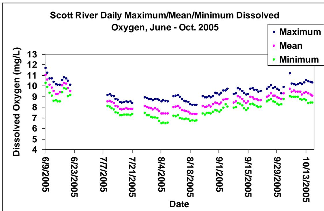
Figure 12. Daily maximum, mean, and minimum dissolved oxygen in the Scott River from June to October, 2005.
