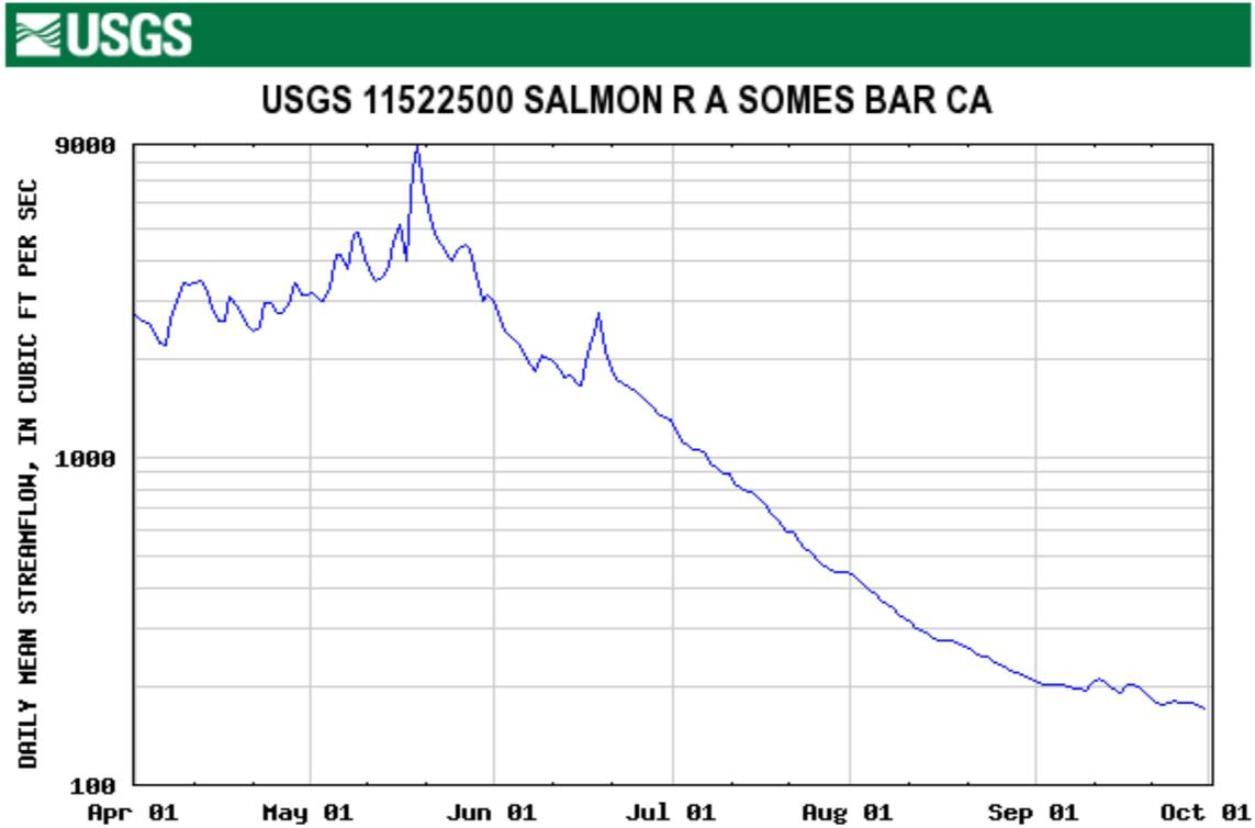
Figure 23. Daily mean stream flow (ft<sup>3</sup>/sec) from the Salmon River at the Somes Bar USGS flow gauge from April to October, 2005.
