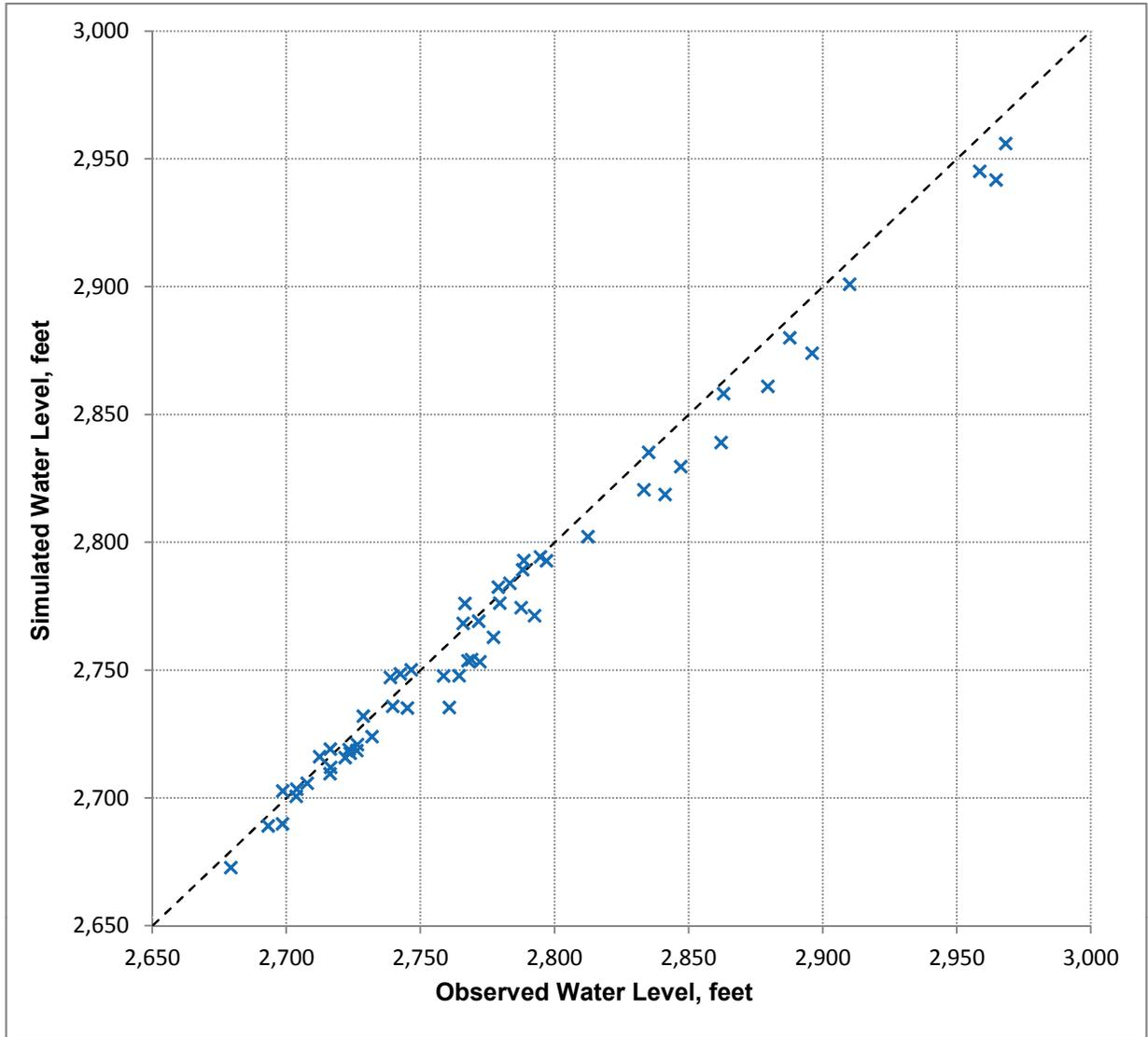
**Figure 5.3 General Comparison of Simulated and Observed Groundwater Elevations**
