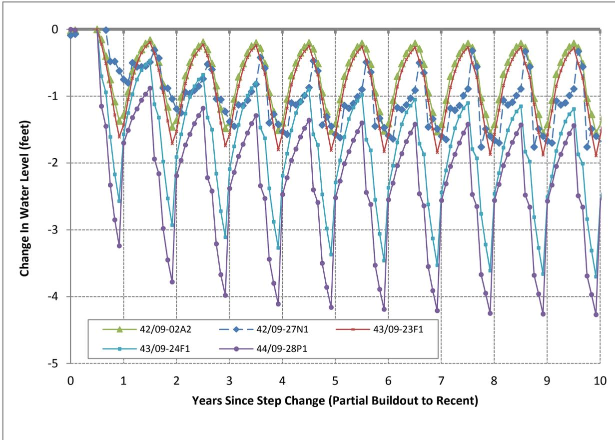
**Figure 6.2 Change in Simulated Groundwater Elevations at Selected Locations due to Step-Change in Pumping from Partial Build-Out to Recent Condition**
