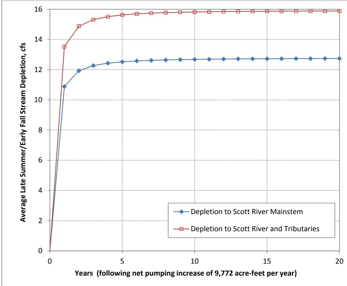
Note: The net increase in pumping is simulated as occurring as a single step; the resulting curve can be used to identify lagged depletion impacts from a gradual change in pumping
