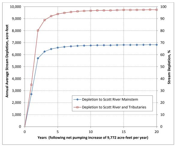
Note: The net increase in pumping is simulated as occurring as a single step; the resulting curve can be used to identify lagged depletion impacts from a gradual change in pumping
