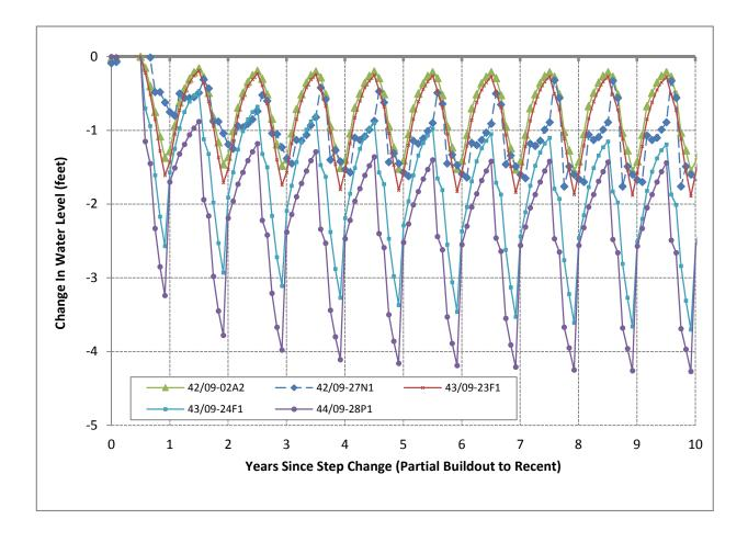
Figure 6.2 Change in Simulated Groundwater Elevations at Selected Locations due to Step-Change in Pumping from Partial Build-Out to Recent Condition
