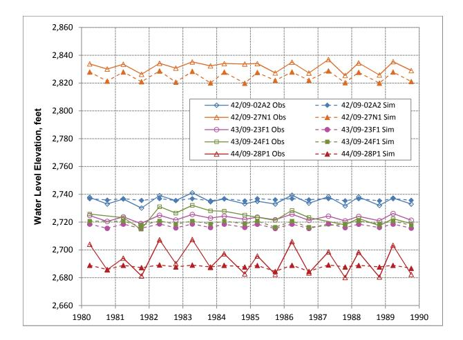
Figure 5.2 Simulated and Observed Groundwater Elevations at Selected Locations, Partial Build-Out
