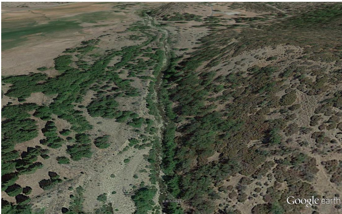
Figure 5. Google Earth image showing the Shasta River approximately 1 mile upstream of I-5. This reach is moderate gradient (~ 2%–3%) slope with predominately cobble substrate and run/step-run mesohabitat.
